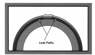
STANDARD CLAMP Leak path may exist from band foldover
