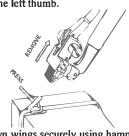
Hammer down wings securely using hammer knob on tensioner, or a similar tool.
