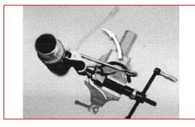
Cut the band with the shear lever.
