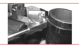
Roll the hose assembly over until the hook of the HBJ001 adapter rests behind the edge of the lock. You must reverse the tension of the tool by 1/2-3/4 of a turn during the roll over process.
