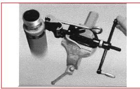
Insert hose assembly into the clamp and apply tension by turning the handle of the tool.
