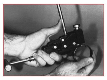
1) Push ball handle forward. This will open the front slot. Insert clamp tail and tension by lifting and lowering tension handle.
