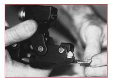
HBC-032 3/8" adapter can be purchased separately and inserted into front of tool for use with 3/8" wide clamps.
