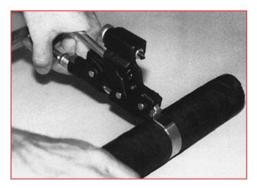
3) Apply forward and backward movements of the tool to break off the clamp tail.
