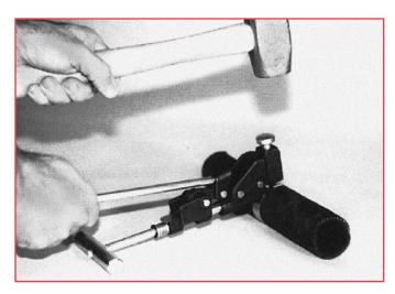
2) When sufficient tension has been reached, secure the clamp by lowering the punch head onto the lock and strike a minimum of 2 times with a 2 lb. mallet.
