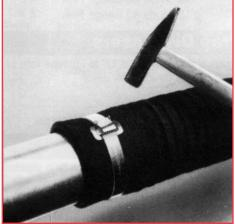
6) While holding the stub of the band with your thumb, hammer flat over bridge of buckle. Complete application by hammering the buckle ears over the stub.
