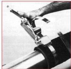
4) When maximum tension has been reached, roll tool over buckle. At same time reversing handle carefully approx. 3/4 turn to avoid breakage. The band that is released will be used in the bend and therefore there is no loss of tension.
